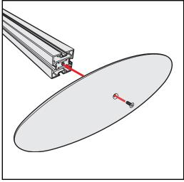
Base Plate & Extrusion Connection
